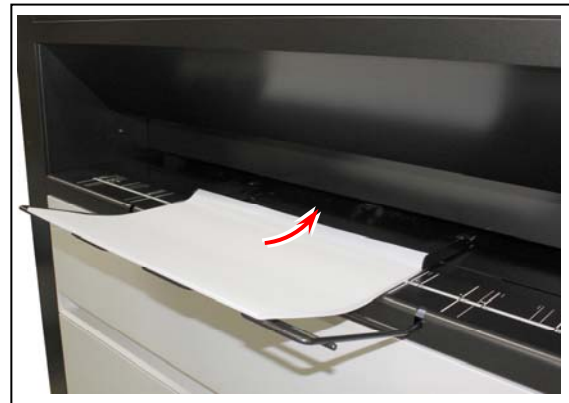
Incorrect (curl up)
