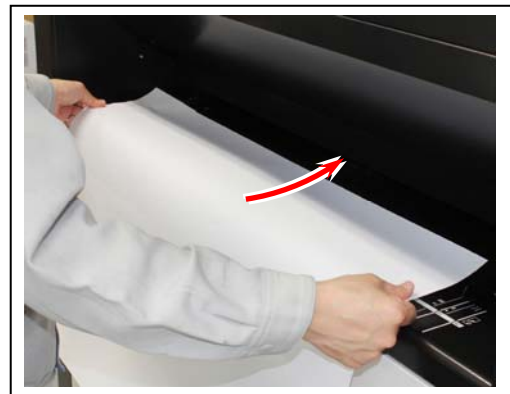
Incorrect (curl up)
